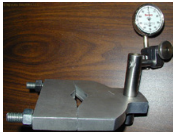
Figure 9. Dial Indicator With Alignment Fixture That Clamps to a Shaft
