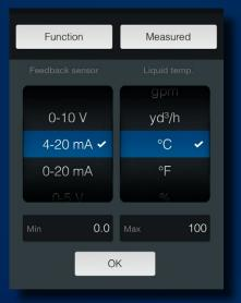
As the TPE3 is fitted with an internal temperature sensor in the pump housing, it only needs one external sensor to operate in ΔT control mode.
