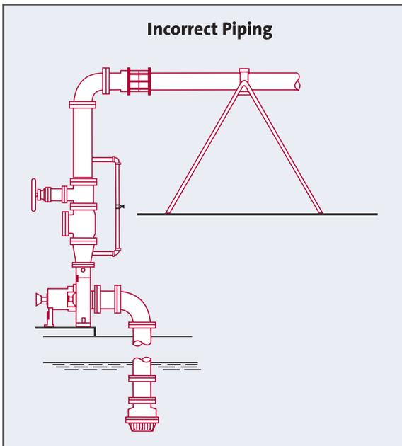
Figure 6. Correct and Incorrect Piping Support
