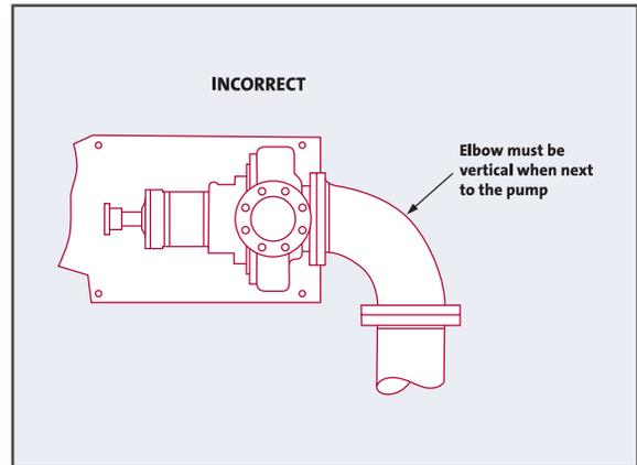
*Figure 4. Incorrect Installation of Elbow*
