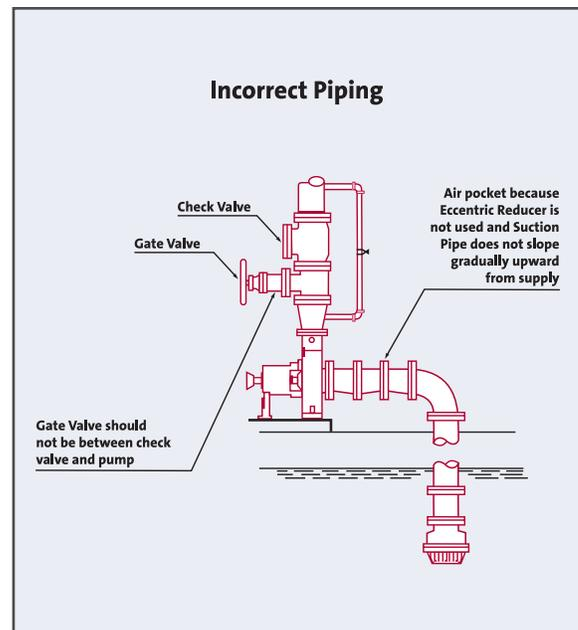
*Figure 5. Correct and Incorrect Piping Configurations*
