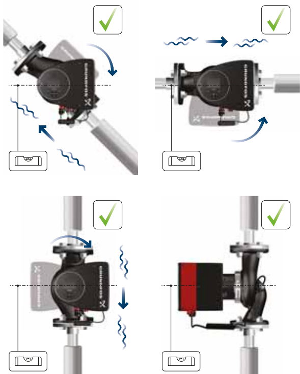
Fig. 7 Pump with the control box in horizontal position
