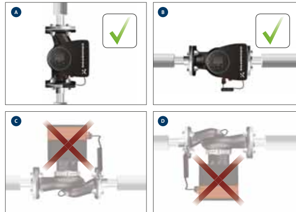
Fig. 6 Pump installed with a horizontal motor shaft
